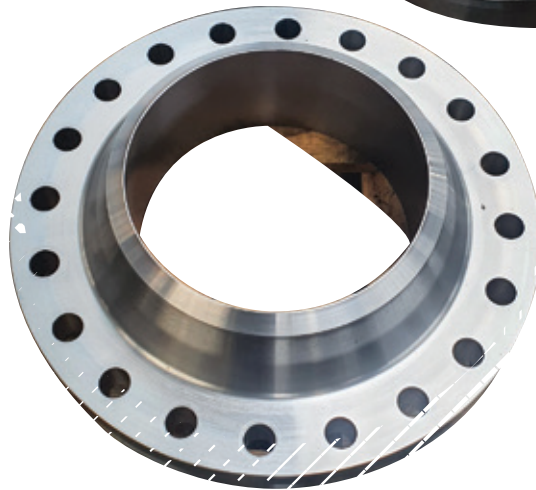
18" 600# WN RJ IN A694 F65 WITH 3MM INTERNAL CLADDING IN INCONEL 625
