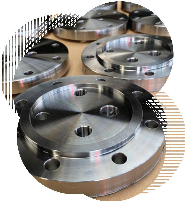
BL. ACC.TO DWG. DIM. 180X26 MM IN F321
